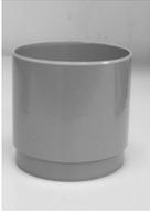
Place the vent inlet coupling into the hole that you have created for the 4" vent so that the 1" of smaller diameter pipe is protruding into the hole in the top of the unit. This is the first piece of the venting. Once you have finished assembling the vent, you should run a bead of silicone around the inlet coupling to prevent odor from escaping.
